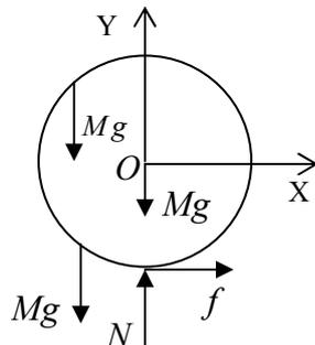
$$\sum F_x = f = 3M \left( \frac{R}{3} \dot{\theta}_0 - \ddot{\theta} R \right) \dots\dots\dots(1)$$
