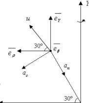
$$\dot{\rho} = (-\omega_2^2 \ r_{AB} \cos 30^\circ) + (2 \ \omega_2 \ u \ sen 30^\circ) = (-0.4^2 * 6 * \cos 30^\circ) + (2 * 0.4 * 0.45 * sen 30^\circ)$$
