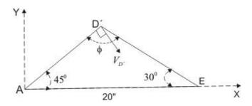
$$\emptyset = 180^{\circ} - 45^{\circ} - 30^{\circ} = 105^{\circ}$$
